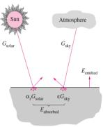
$$q_{net,rad} = \alpha_s G_{solar} + \varepsilon \sigma (T_{sky}^4 - T_s^4) [W/m^2]$$
