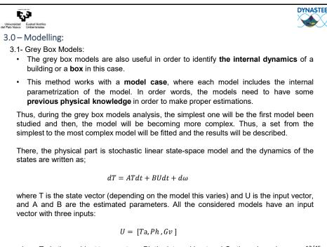
where Ta is the ambient temperatura, Ph the internal heat and Gv the solar gains.
