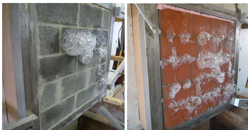
Figure 3. Visualization of air leakage by means of a soap/water solution during the determination of the air permeability of a concrete wall
