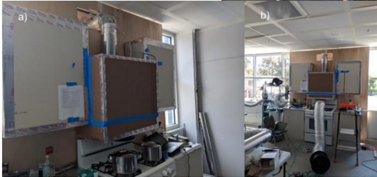
About 15% of flow missed if measurements are made for the bottom inlet only
