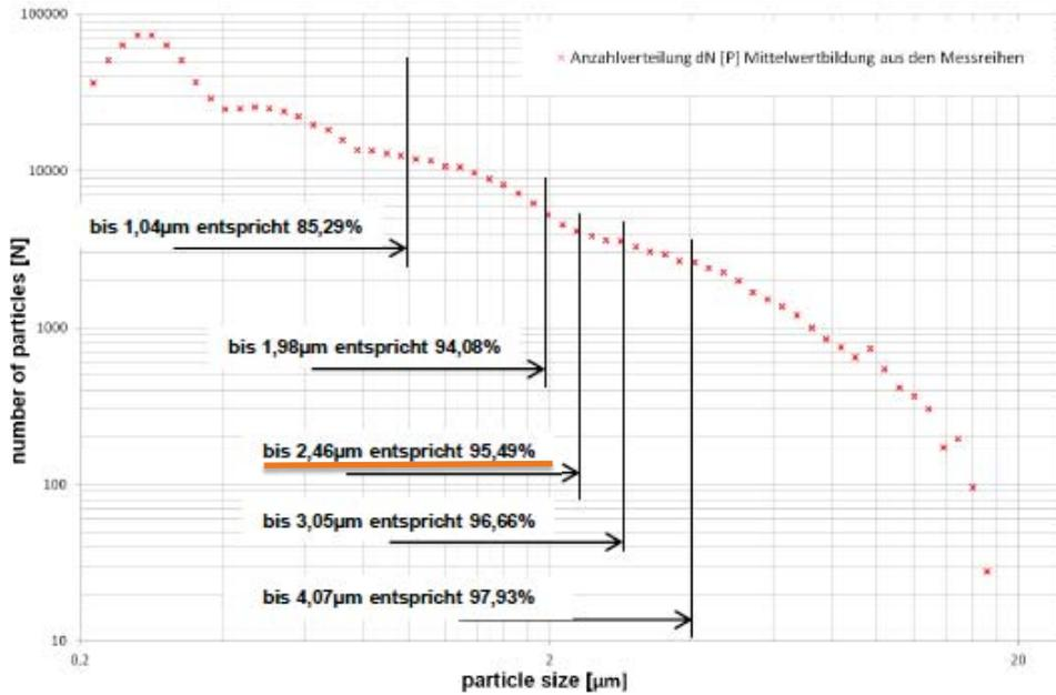
=> Particles smaller 2,5 µm represent more than 95% of particle amount
