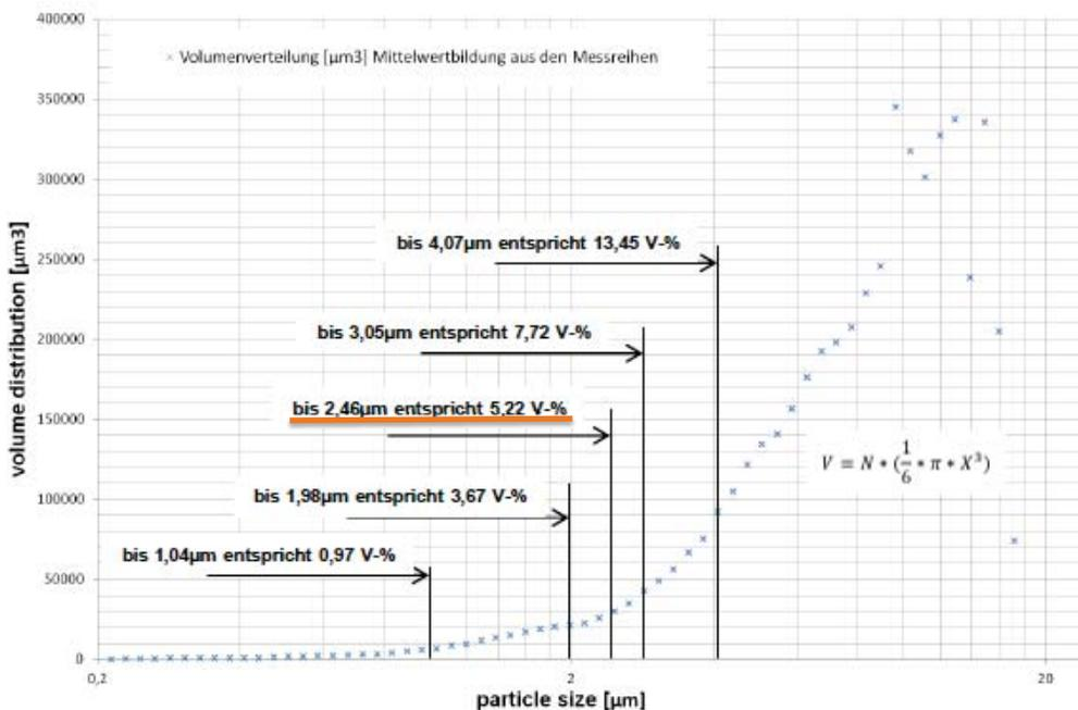
=> Particles smaller 2,5 µm correspond to 5,5% of particle mass
