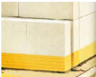
Puren insulation bridge under the first row of masonry to reduce the thermal bridge impact [Copyright Puren GmbH].
