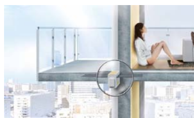
Section drawing showing how an Isokorb is forming a thermal break between the building and the balcony [Copyright Schöck Bauteile GmbH].
