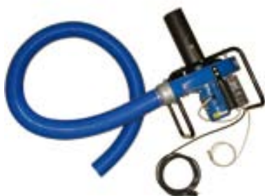
Fig.26 Example of Scandinavian duct leakage testing equipment [Swema]
