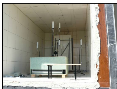
(1) Interior of PASLINK renovated test-cell with HeatFlow sensor tiles
