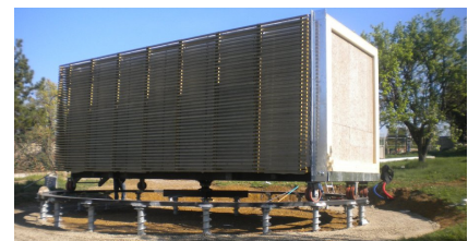
New design of PASLINK testcell in Florence
