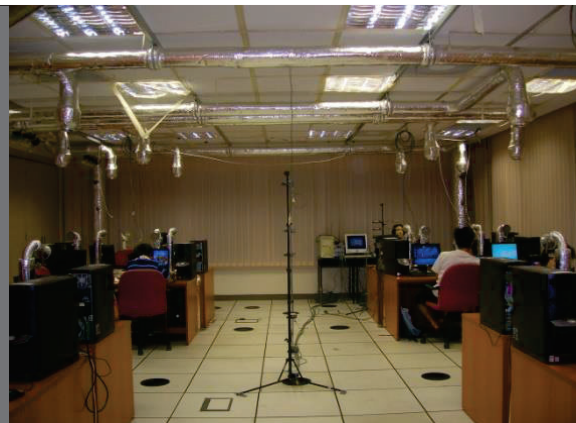
Field Environmental Chamber (FEC) experimental setup - Desk mounted PV with UFAD system
