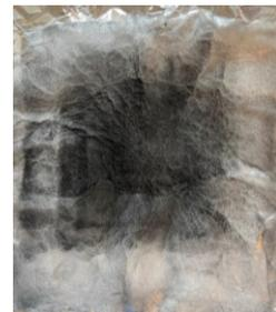
AC sprayed on the CA filter
