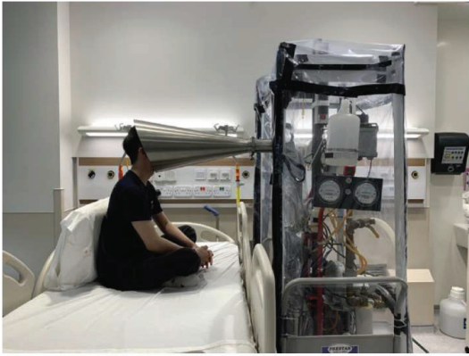
Figure 1. Schematic representation of expiratory sample collection using the G-II exhaled breath collector inside the COVID-19 patient room. Abbreviation: COVID-19, coronavirus disease 2019.
