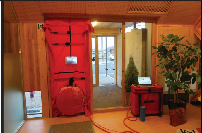
Blower Door Test, twice
