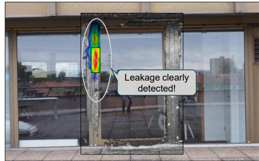
Combination of infrared and acoustic camera
