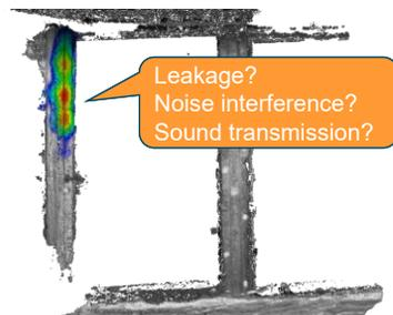
3D model of the acoustic camera with sound localization
