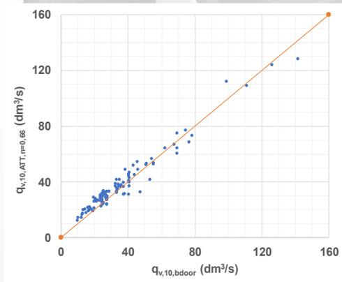
Koppen bouwexperts is a specialist in the field of air tightness measurements with the blower door. In 2018 and 2019, they compared the ATT with the blower door in a large number of homes.
