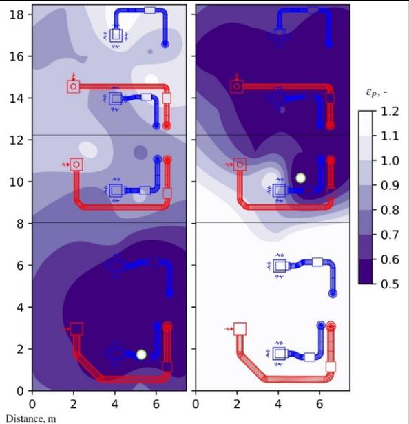
Large teaching space of 130 m<sup>2</sup> with 4 L/(s m<sup>2</sup>) ventilation:  $\epsilon_b^1=0.76$  (left) and  $\epsilon_b^2=0.77$  (right) and the average value of two measurements  $\epsilon_b=0.76$
