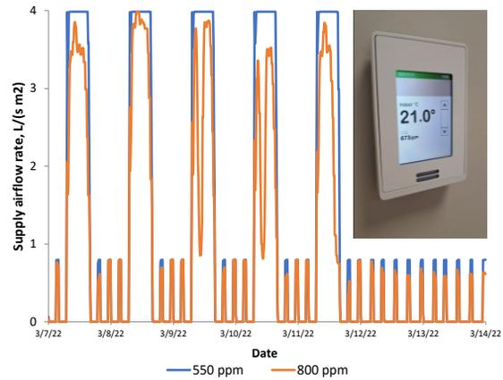
Ventilation airflow rates in a typical classroom with CO<sub>2</sub> set point of 550 ppm and 800 ppm
