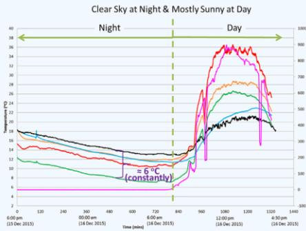
Fig. 10. Temperature profile of the passive radiative coolers under a clear night sky weather condition.
