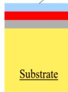
**Mid layer:** Solar reflective component - layer 1: non-thermal emitter (fluorescent) material (white/metallic or non-white/non-metallic) with fluorescence in (300 nm- $\lambda_{\text{AE}}$ ) and high light transmission in ( $\lambda_{\text{AE}}$ -2500 nm)
