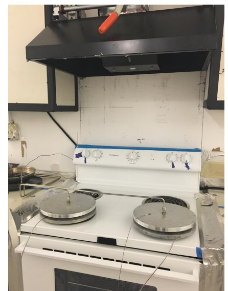
Emitter plates on cooktop during Capture Efficiency Testing
