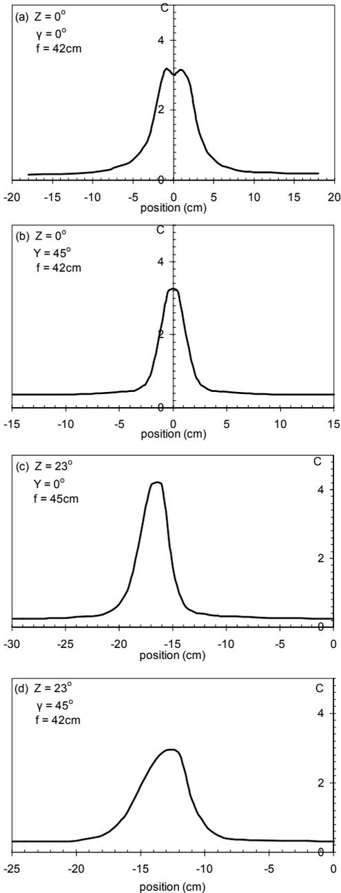
Figure 2: Diagrams showing the distribution of concentrated solar radiation by the used fresnel lens.
