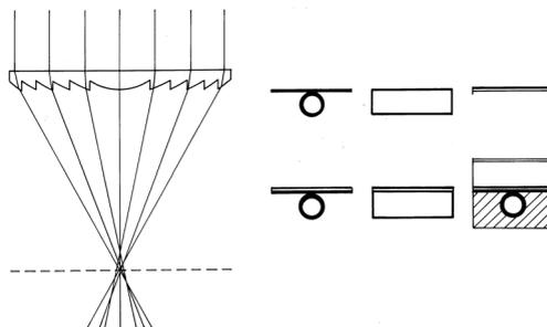
Figure 1: The geometry of the linear Fresnel lens, with indication of the concentrating solar radiation (left) and alternative absorbers of Thermal (T), PV and PVT type (right).
