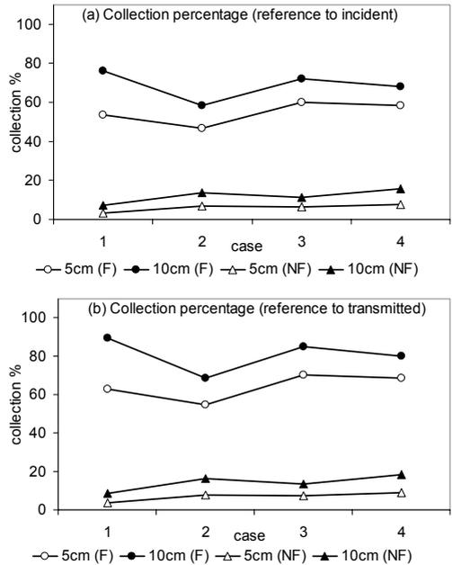
Figure 3: Collected solar radiation for the cases of Fig. 2 and absorbers (5cm, 10cm) in focus (F) or no focus (NF).
