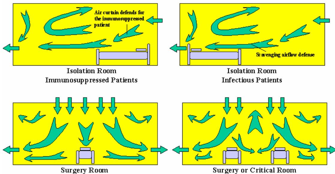
Figure 2: Airflow Configurations for Critical Areas
