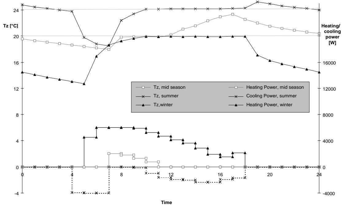
Fig. 4 : Three typical days, optimal temperature and heating/cooling profiles
