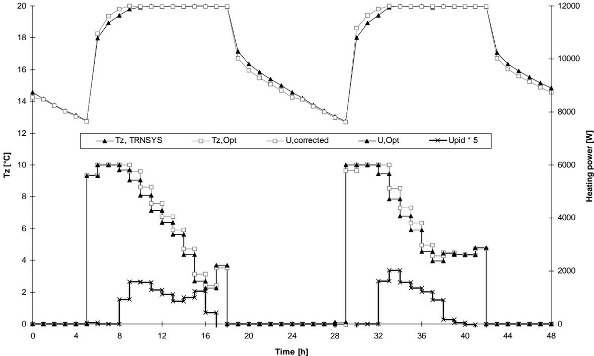
Fig. 6 : Optimal temperature and control signal and PID correction
