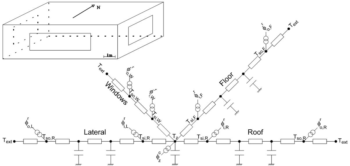
Fig. 2 : The example thermal zone and its simplified model
