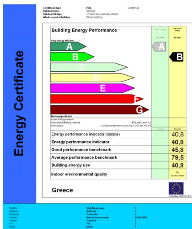
Figure 1: Preliminary design of the energy certificate proposed by the EP label approach.
