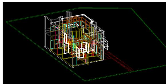
The three-dimensional model of an existing historical building that is a celebrated example of De Stijl architecture (Figure 1) was displayed by one CAD program and slightly modified. The modified, IFC-compliant CAD file was then sent to another CAD
