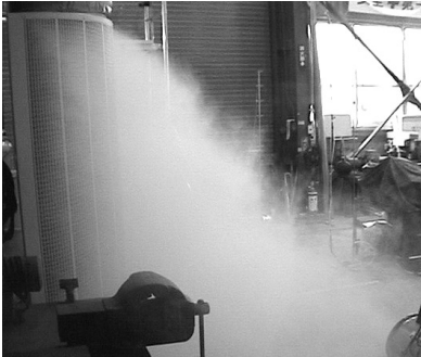
Photo. 1. Airflow pattern of the DV
