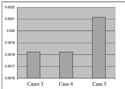
Figure 13 The fraction of contaminant mass flow rate leaking from the hood to the room against the contaminant mass removed by the hood exhausts for Cases 3-5
