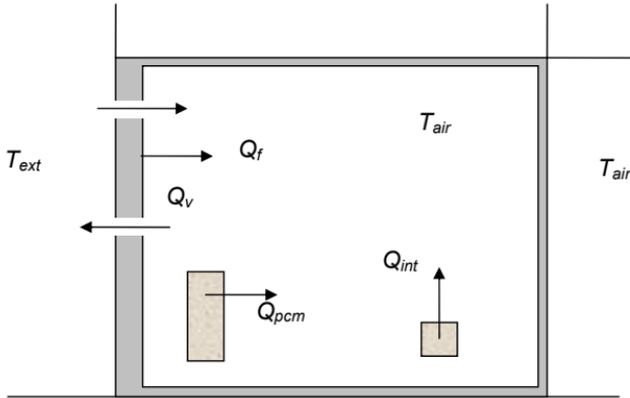
Figure 1. Basic configuration used for simulation
