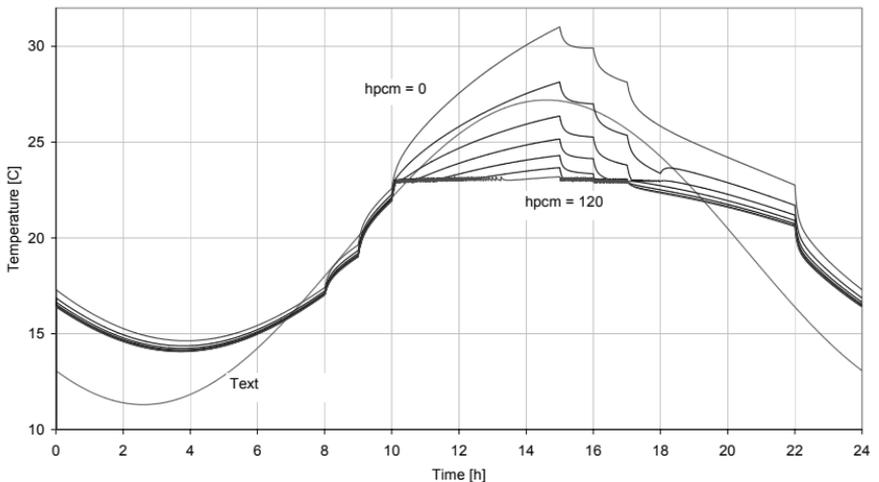
Figure 5. Effect of increasing heat transfer coefficient from 0 to  $120 \text{ W/K}$  ( $E_{pcm} = 2.5 \text{ kWh}$ )
