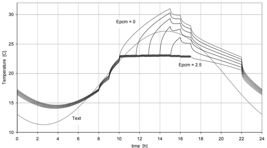
Figure 4. Effect of increasing storage capacity from 0 to 2.5 kWh in 0.5 kWh steps ( $h_{pcm} = 120$  W/K)
