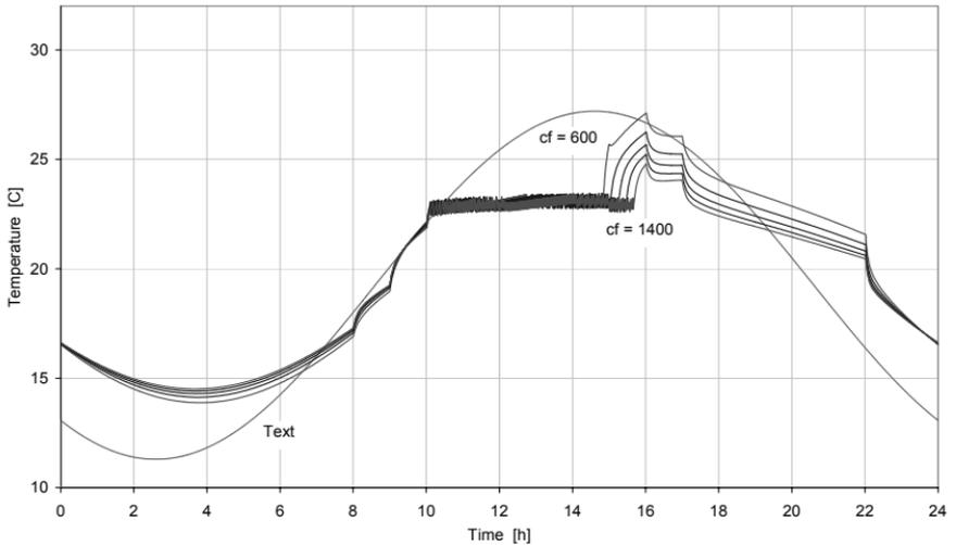
Figure 6. Effect of increasing specific heat capacity of fabric from 600 to 1400 J/kgK
