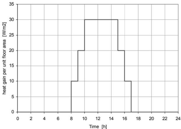
Figure 3. Example of variation of internal heat gain with time
