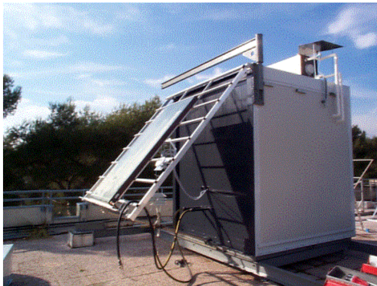
Figure 1. The automatic test bench for solar collectors in Sophia-Antipolis.
