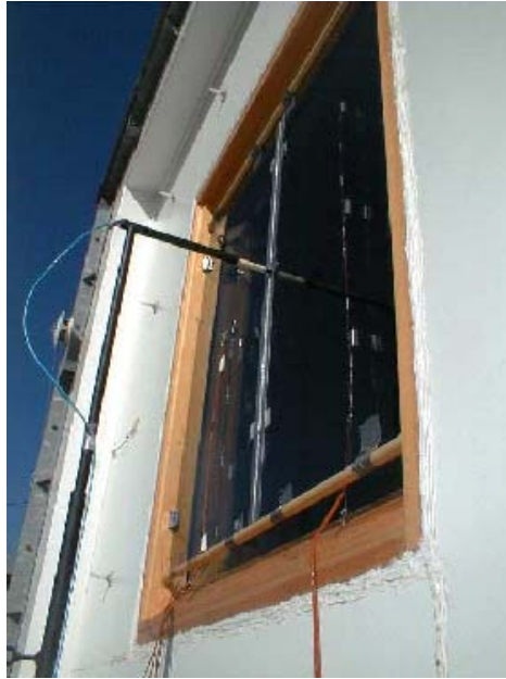
Figure 2. Prototype of the SOLVENT window mounted on the PASSYS test cell in Summer mode.
