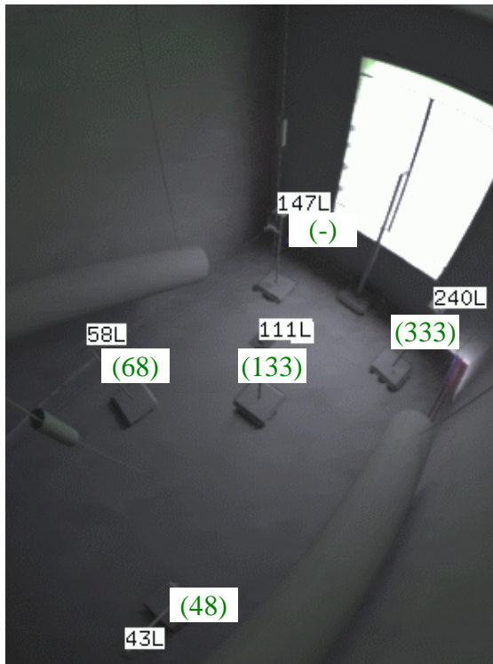
Figure 15a. Simulated illuminance levels under overcast sky conditions and measured values on 5 th October at 12:00 (measured values between brackets).
