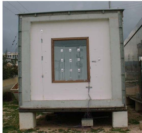
Figure 3. The window installed in the opaque surround at BRE, Scotland, and CRES, Greece.
